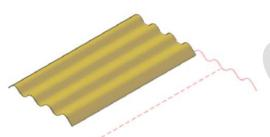
The path curve can be a line, arc, circle, ellipse, elliptical arc, 2D polyline, 3D polyline, or spline. The direction vector can be based on a line or an open 2D or 3D polyline.
